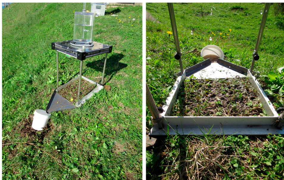
Figure 3. Rain simulator operating in one of the experimental plots (Locri, Southern Italy).
